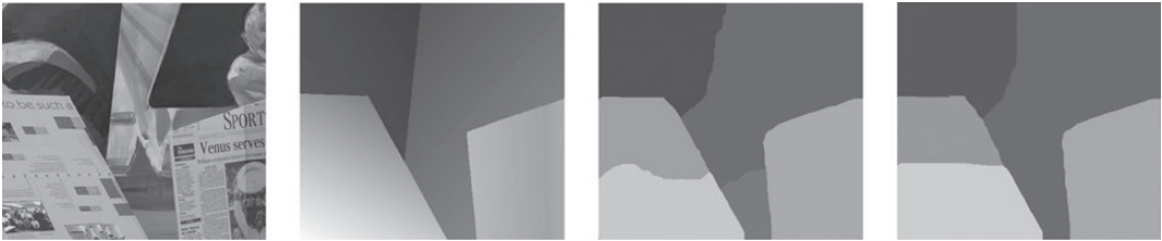
FIG. 2. Results for the images 'Venus'. Left to right: original left image, ground truth, partitioned disparity using the two-stage algorithm ( \alpha_1 = 0.005 , \alpha_2 = 300 ), partitioned disparity using the direct algorithm ( \lambda = 2.5 ) (source: http://vision.middlebury.edu/stereo/ . Last accessed December 12, 2014 [54]).
