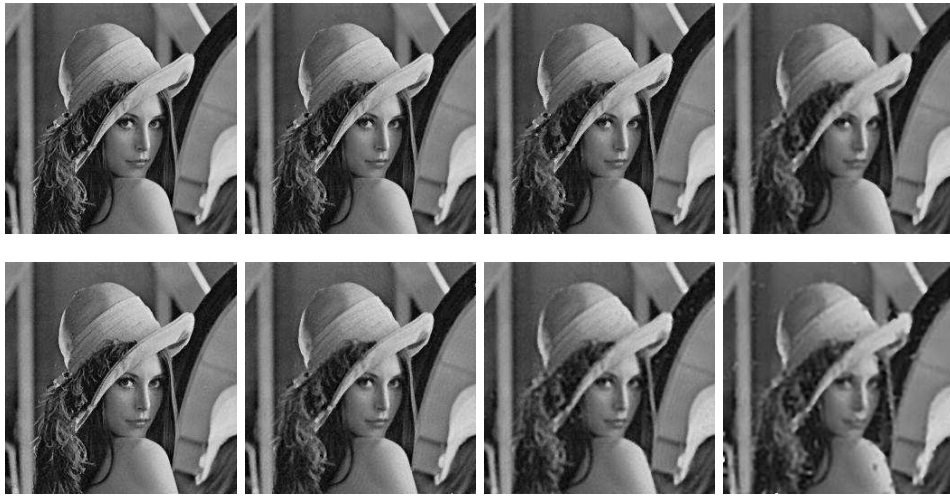
FIGURE 8. Lena image blurred with out-of-focus kernel of radius 3, and then corrupted by random-valued noise with noise levels are 10%, 25%, 40%, and 55% respectively. Top : The restored image by our method, and the parameters we used are [\alpha = 0.0005, \beta = 0.0005, \epsilon = 0.001] , [\alpha = 0.001, \beta = 0.001, \epsilon = 0.0005] , [\alpha = 0.002, \beta = 0.002, \epsilon = 0.0005] , [\alpha = 0.005, \beta = 0.005, \epsilon = 0.0001] respectively. Bottom : The restored image by the full variational method, and the parameters we used are [\alpha = 0.001, \beta = 0.001, \epsilon = 0.0005] , [\alpha = 0.005, \beta = 0.005, \epsilon = 0.0005] , [\alpha = 0.005, \beta = 0.005, \epsilon = 0.00005] , [\alpha = 0.01, \beta = 0.01, \epsilon = 0.0001] respectively.
