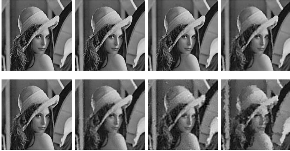
FIGURE 4. Lena image blurred with out-of-focus kernel of radius 3, and then corrupted by salt-and-pepper noise with noise levels 30%, 50%, 70%, and 90% respectively. Top : The restored image by our method, and the parameters we used are [\alpha = 0.0002, \beta = 0.0002, \epsilon = 0.001] , [\alpha = 0.0002, \beta = 0.0002, \epsilon = 0.0005] , [\alpha = 0.0005, \beta = 0.0005, \epsilon = 0.0002] , [\alpha = 0.001, \beta = 0.001, \epsilon = 0.0001] respectively. Bottom : The restored image by the full variational method [4, 5, 6], and the parameters we used are [\alpha = 0.005, \beta = 0.002, \epsilon = 0.0002] , [\alpha = 0.01, \beta = 0.01, \epsilon = 0.0001] , [\alpha = 0.01, \beta = 0.01, \epsilon = 0.00005] , [\alpha = 0.01, \beta = 0.01, \epsilon = 0.00005] respectively.
