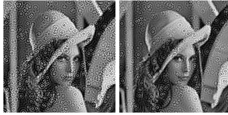
FIGURE 2. Lena image blurred with out-of-focus kernel of radius 3, and then corrupted by impulse noise. The image is restored by minimizing (3)–(4) with \varphi(t) = \sqrt{t^2 + 10^{-4}} and \beta = 0.01 . The left is the restored image when s = 1\% and the right is when r = 1\% .
