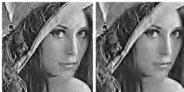
(a) Translation invariant wavelet thresholding ( T = 50 ) (b) Fast method adapted to translation invariant wavelets
